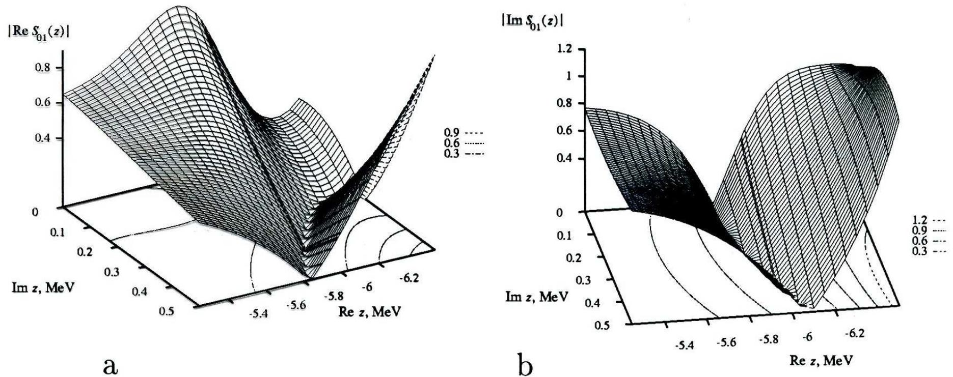
FIG. 3. Surface of the absolute values of real (a) and imaginary (b) components of the scattering matrix  $S_{01}(z)$  in the model system of three bosons with the nucleon masses.
