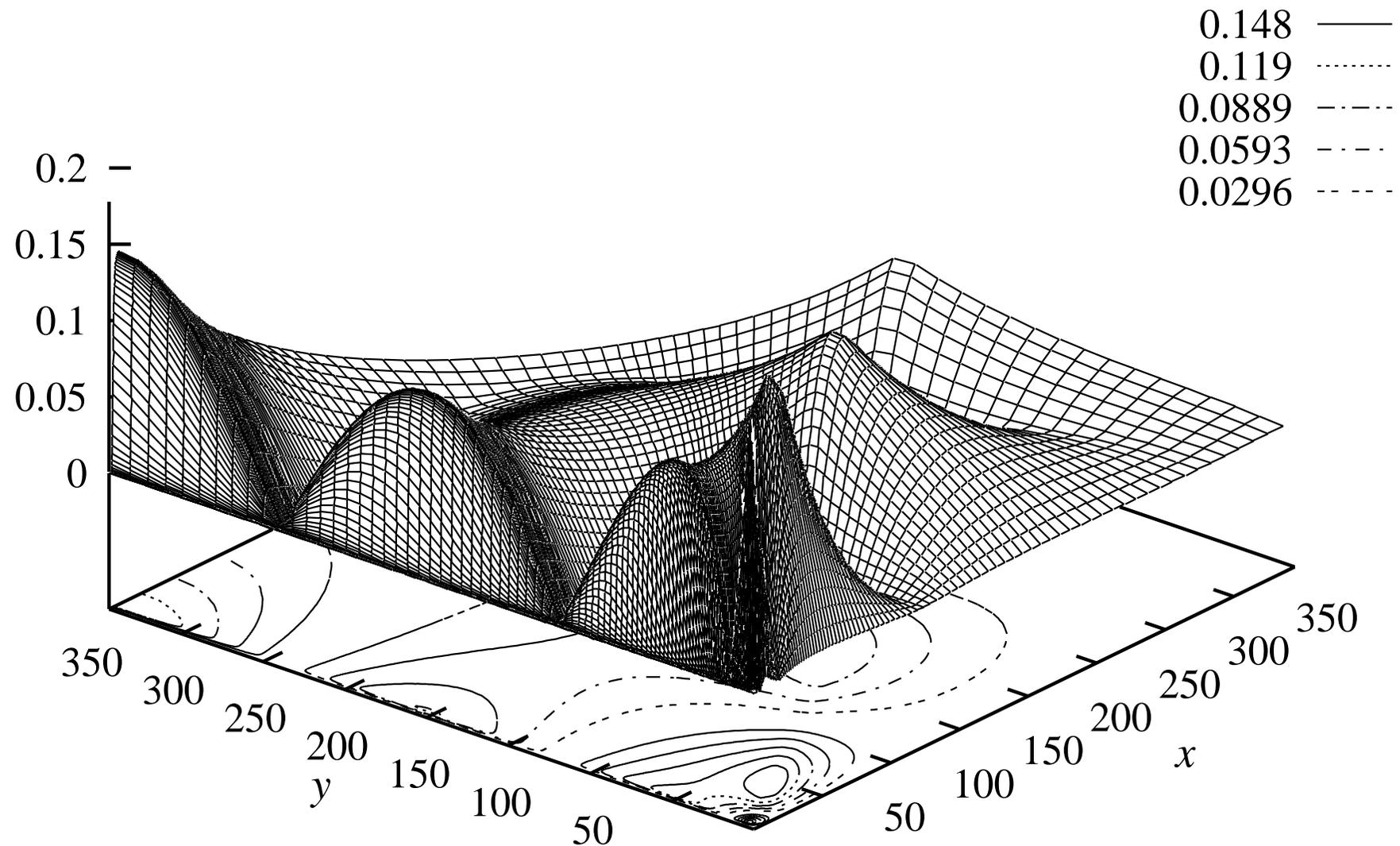
Absolute value of the  ${}^4\text{He}-{}^4\text{He}_2$  scattering wave function component  $\Psi_0(x, y, p)$  for the HFD-B  ${}^4\text{He}-{}^4\text{He}$  potential at  $E = +1.4$  mK.
