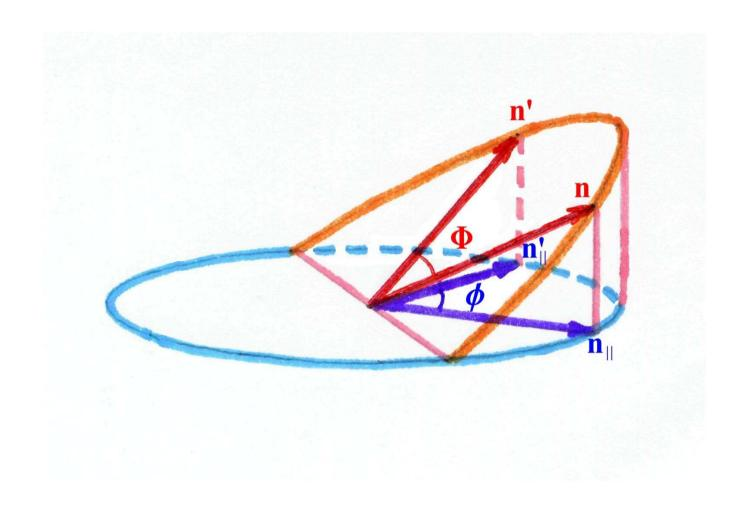
The angle  $\Phi$  between two positions of rotating vector N in the tilted plane is not equal to the angle  $\phi$  between two corresponding horizontal projections. Therefore, the vertical betatron oscillations
